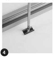
Fix clips with to surface with suitable screws (min. 2 per metre/40"). Mark & drill holes if required.
